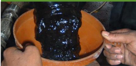
Sludge from petroleum refinery introduced in the SUSTECH machine
